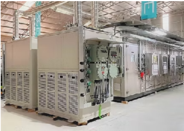
ADAGE Integrated Solution Analyzer Shelters for Zone 1 & Zone 2 applications with HVAC In-house Design and Manufacturing facility for SS316 /304.
